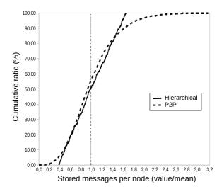
Fig. 3. Load balancing with random inserts
