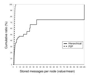
Fig. 4. Load balancing with Zipf distribution based inserts
