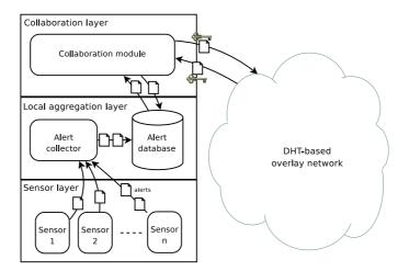
Fig. 2. Design of a collaborative alert aggregator
