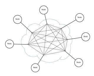
Fig. 1. Node connections to the DHT
